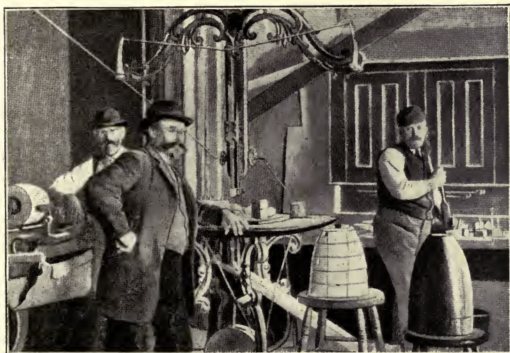
PLATE 4.—Chiselling and turning blocks of gun-cotton for charging shells. The brass-nose shell is shown on the right-hand stool, and the charge for this on the left-hand stool and in the lathe.
